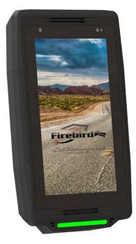
The Firebird Vehicle-Mounted Computer fills a void in the market for affordable, yet durable, forklift mounted devices. The Firebird is sized right to provide the user with a large 7" screen to keep task-related data easily viewable, yet not impeding the field of view when driving the vehicle, a critically important safety feature.
