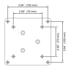
The KDT3 includes the VESA 75 standard for mounting. The four mounting holes are centered left-to-right on the upper portion of the back panel. These holes are exactly 75mm x 75mm on center and accept the standard 4mm screw.
