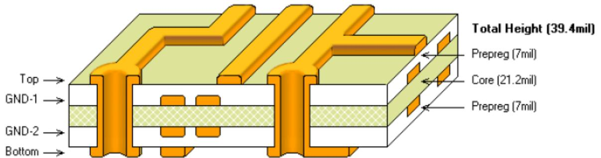
Figure 8 PCB layer stack-up for multi-layer board (Example)
