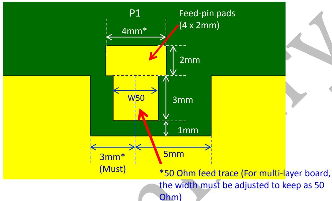
**Figure 7** Airgain N703LTSTM antenna feed trace layout requirement
