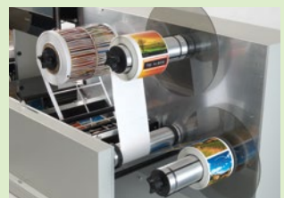
Rewinding to finished rolls
