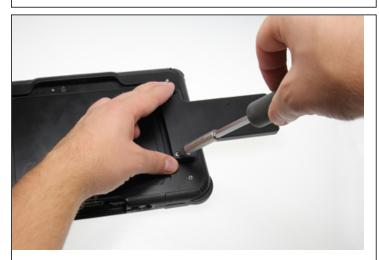
3. Secure the Extension Plate using the enclosed machine screws.
