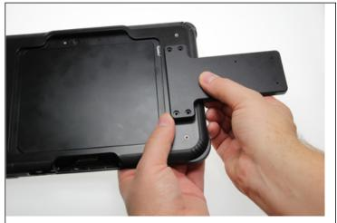
2. Place the Extension Plate over the matching holes in the ET5X Rugged Frame.
