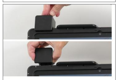
3. Using the Spring Lock The spring lock can be slid down and over the top of the tablet after it is docked. This provides additional protection from vibration that occurs front to back in more rugged environments.
