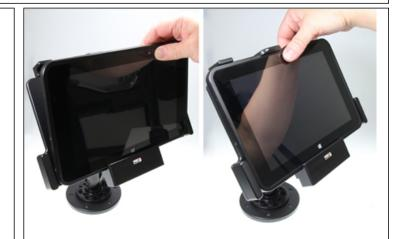
2. To place the device in the cradle: Place the lower part of the device in the cradle, then flip/press the upper part forwards so it snaps into place in the cradle.
