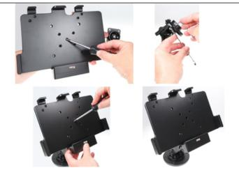
1. Unscrew the screw in the center of the cradle so you can remove the tilt swivel base plate on the back. Place the base plate over the matching holes in the face plate of your mounting bracket (ProClip aluminum pedestal shown in picture) Attach the base plate by using the applicable bolts enclosed. Place the cradle onto the tilt swivel base plate and attach it with the center screw.
