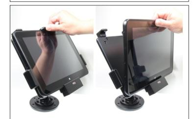
3. To remove the tablet from the cradle: Press upwards on the upper part of the cradle, in the same time pull the upper part of the device out from the cradleand then lift the device up and out from the cradle.
