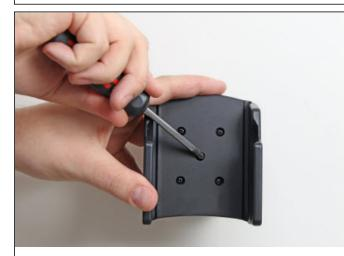
3. Place the holder onto the tilt swivel base plate and reattach it with the center screw. The center screw also controls the pivot, tighter for a firm hold and loose for easier rotation/angling of the Holder.
