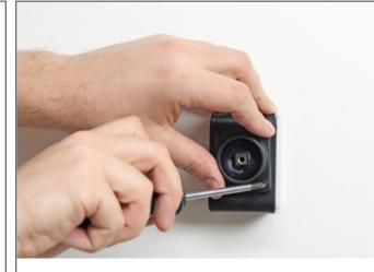
2. Place the Tilt Swivel base plate over the matching holes in your mounting bracket (demo ProClip mount shown in picture). Attach the base plate by using the applicable screws enclosed - self-tapping screws if the mount has small holes or machine screws with nuts if the mount has larger holes.
