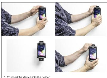
3. To insert the device into the holder: Slide the device down into the holder.
