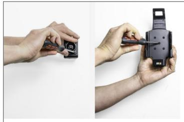
2. Place the Tilt Swivel base plate over the matching holes in your mounting bracket (demo ProClip mount shown in picture). Attach the base plate by using the applicable screws enclosed - self-tapping screws if the mount has small holes or machine screws with nuts if the mount has larger holes.
