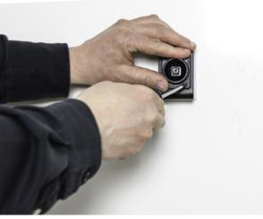
2. Place the Tilt Swivel base plate over the matching holes in your mounting bracket (demo ProClip mount shown in picture). Attach the base plate by using the applicable screws enclosed - self-tapping screws if the mount has small holes or machine screws with nuts if the mount has larger holes.
