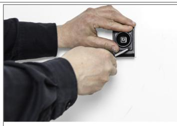
2. Place the Tilt Swivel base plate over the matching holes in your mounting bracket (demo ProClip mount shown in picture). Attach the base plate by using the applicable screws enclosed - self-tapping screws if the mount has small holes or machine screws with nuts if the mount has larger holes.
