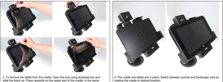
3. To remove the tablet from the cradle: Open the lock using enclosed key and slide the block up. Press upwards on the upper part of the cradle, in the same time pull the upper part of the device out from the cradle and then lift the device up and out from the cradle.
