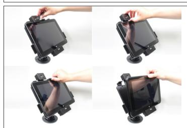
3. To remove the tablet from the cradle: Open the lock using enclosed key and slide the block up. Press upwards on the upper part of the cradle, in the same time pull the upper part of the device out from the cradle and then lift the device up and out from the cradle.
