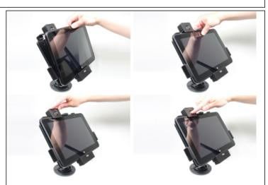
2. To place the device in the cradle: Place the lower part of the device in the cradle, then flip/press the upper part forwards so it snaps into place in the cradle. Slide the key lock into place and press the lock button to secure.
