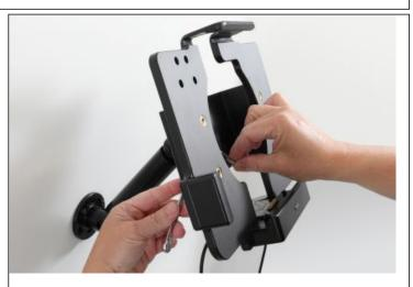
2. **Mounting the Cradle:**This cradle features the AMPS and VESA75 hole pattern in the steel base plate. AMPS is common for many ball and vehicle mounts and VESA75 is common in telecommunications and office environments.
