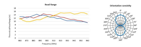
All the graphs are indicative: performance in real life applications may vary. The data has been determined based on calculations for transmitters with a 2W ERP output power level and an NXP Ucode 8 tag silicon.
