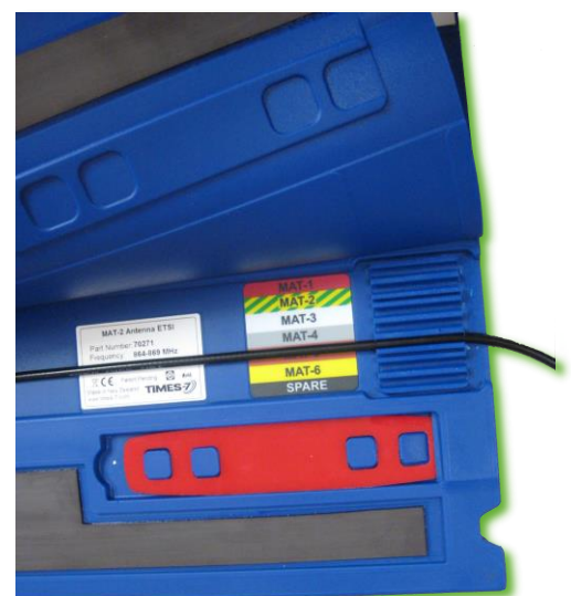
Integrated cable channels – Cable detail
