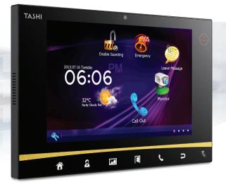
The MT880 is an IP Master Controller designed for both home and enterprise use. Featuring high speed ethernet, wireless communication, and a large capacitive multi-touch screen, the MT880 is equipped with Elfin software to streamline the smart home or office.
