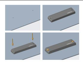
Instructions for optimal performances: 1.Drill two holes on the subject metal surface. [ø 4.0 mm], picth: 65.7mm] 2.Insert two  $\phi 3.4 mm$  (recommended size) rivets on the tag. 3.Fix the tag on the metal surface with a rivet gun.
